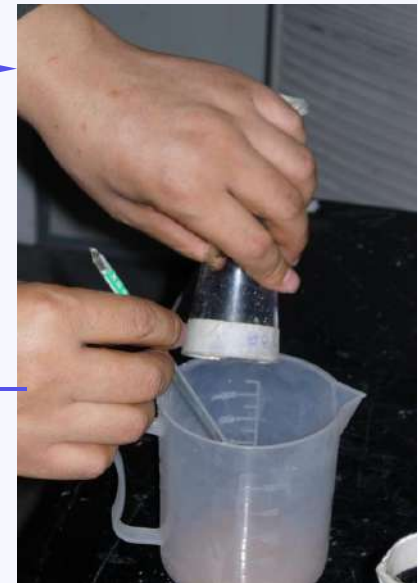
Desiccant temperature rise test \Delta T > 30^{\circ}\text{C}
