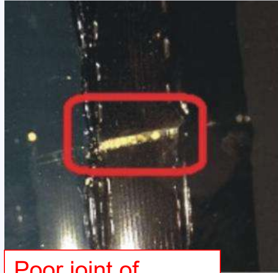
poor overlap of low- e and butyl
