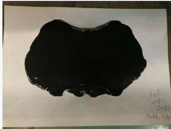
Snap test and Butterfly Test for silicone sealant
