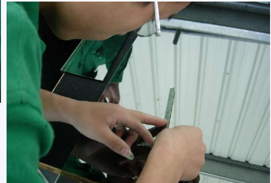
Visual check: Measuring length of scratch 目视检查：测量划伤的长度
