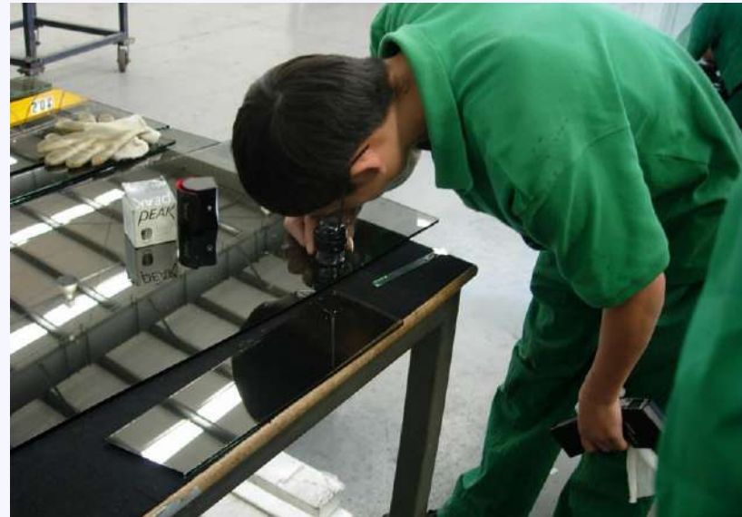
Visual check: Pinhole, Scratches, Streaks, Splotches 目视检查：针孔、划伤、色带、斑点
