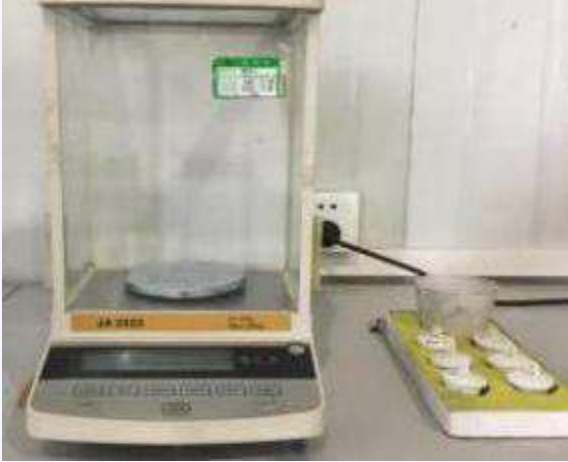
Water initial content measuring for desiccant
