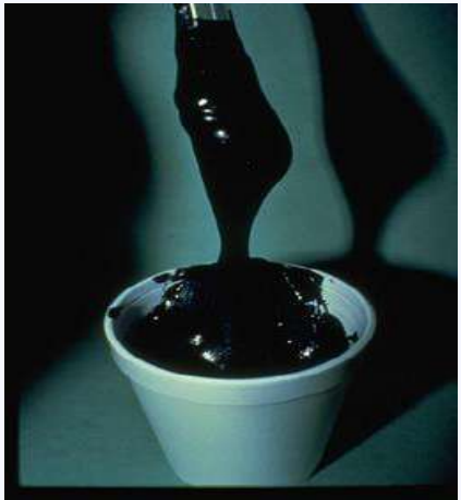
Snap test and Butterfly Test for silicone sealant
