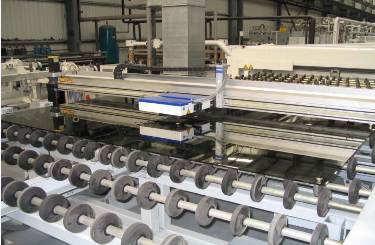
Color control by online color scanner 通过在线颜色扫描仪监控颜色
