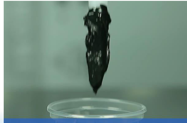
Snap time test: check curing time
